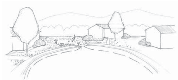
Bioretention facility configured and planted as a lawn/ play area.
